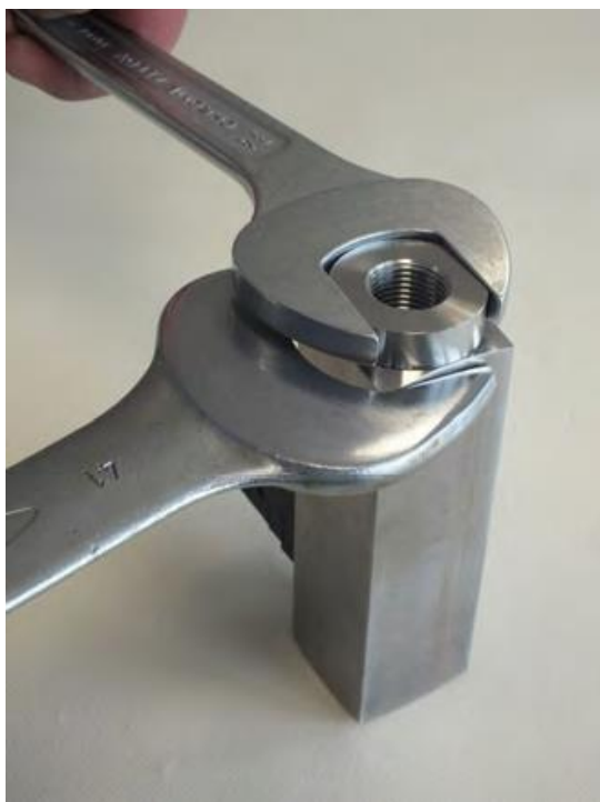
Fig. 51: Tighten process connection (inlet)
