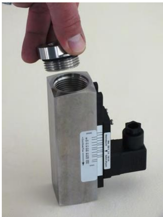
Fig. 50: Insert process connection (inlet)
