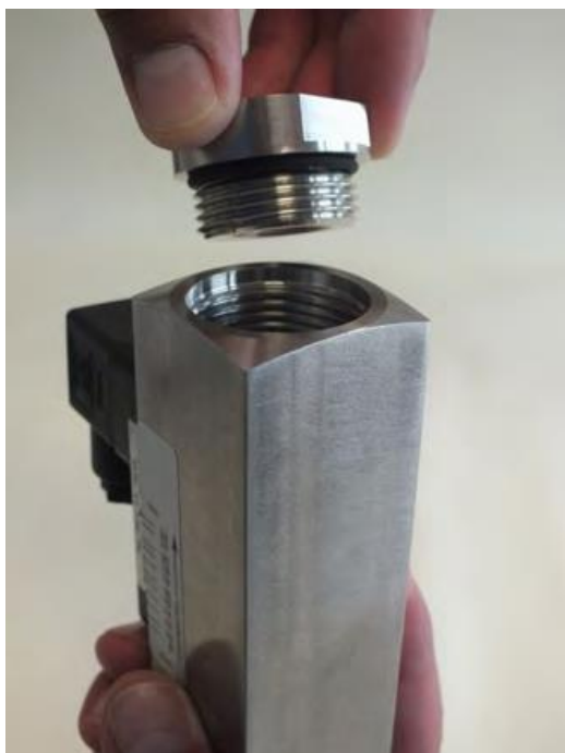
Fig. 35: Remove the process connection (outlet)
