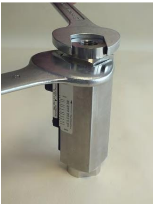
Fig. 34: Loosen process connection (outlet)
