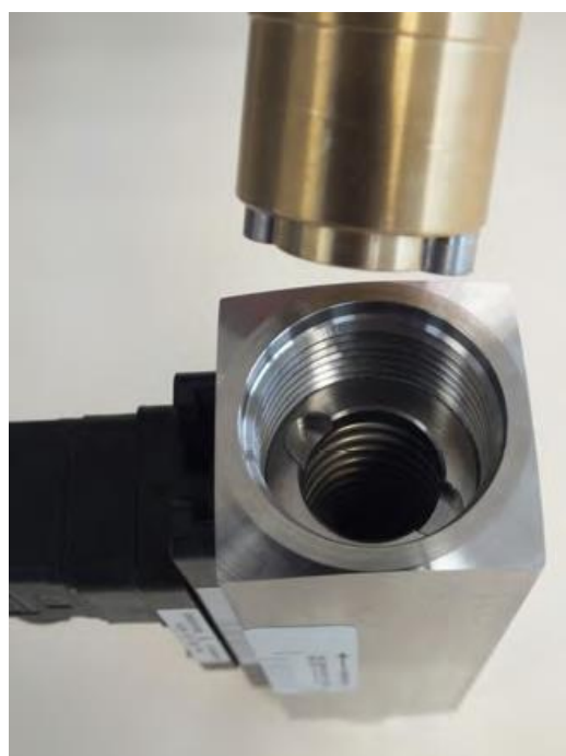
Fig. 36: Insert threaded ring insertion tool (outlet)
