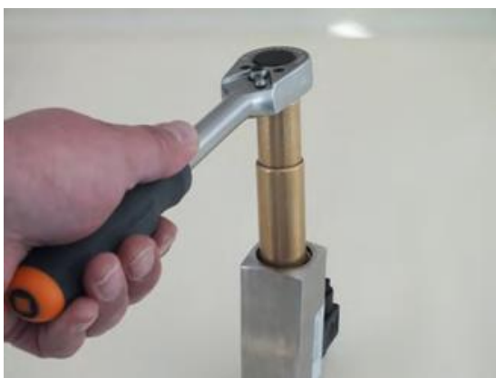
Fig. 49: Seat threaded ring (inlet)
