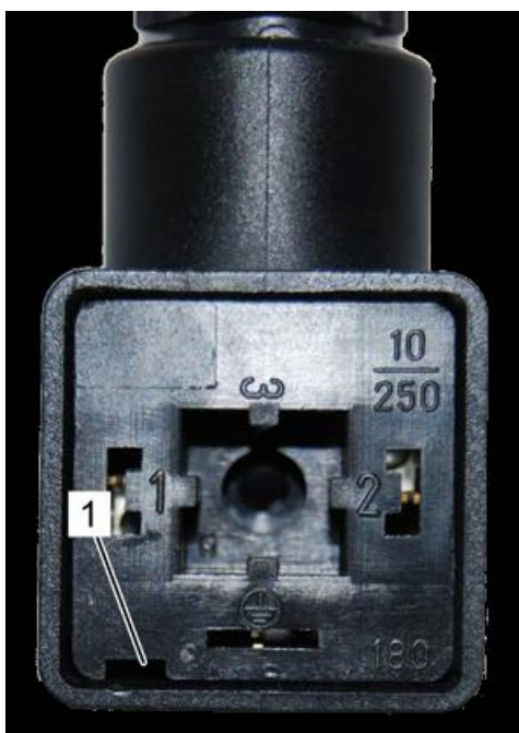
Fig. 22: Disconnect inner section
