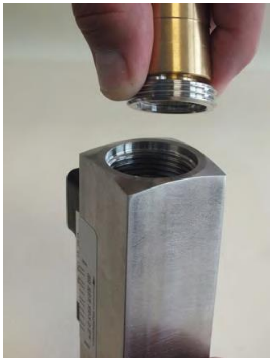
Fig. 38: Remove threaded ring (outlet)
