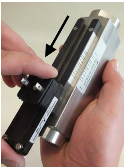
Fig. 62 Remove switch contact from guide rails
