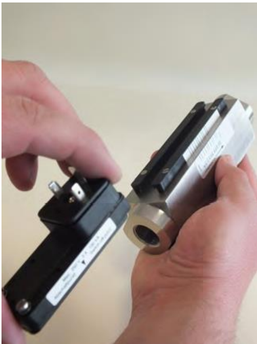
Fig. 63: Remove switch contact
