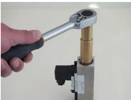
Fig. 37: Loosen threaded ring (outlet)
