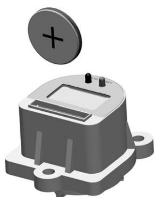
2. Fit the supplied CR2032 battery as illustrated and push it firmly down.
