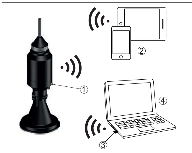
Fig. 4: Wireless connection to standard operating devices
