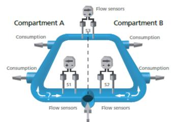
Consumption compartment A (m<sup>3</sup>): Vol S1 (m<sup>3</sup>) - Vol S3 (m<sup>3</sup>) Consumption compartment B (m<sup>3</sup>): Vol S2 (m<sup>3</sup>) + Vol S3 (m<sup>3</sup>)
